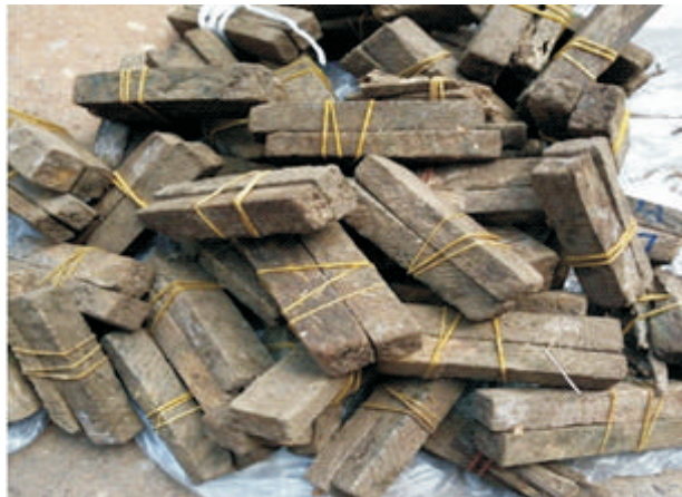
Plate 11: Test Wood samples after exposure to Termite
